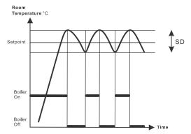
PID intelligent learning control algorithm periodically switches on and off the heating system. The period time (T) and pulse length (P) of the control signal (PWM) are determined by the setpoint and the measured room temperature.
