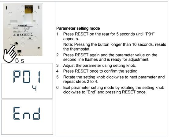
Note: The thermostat automatically exits parameter setting mode one minute after the last action.
